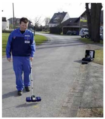
The Wohler VIS 350 precisely locates radio waves transmitted by the camera head through concrete and asphalt to save a lot of time and further building damage.
