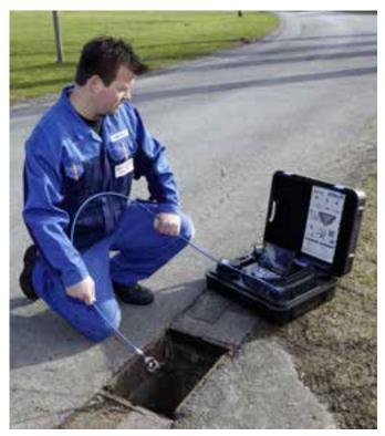
The 100 ft. push rod and the pan&tilt color camera head make sure nothing in the house supply line remains hidden from your view.
