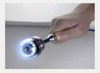
Thanks to the excellent lighting system of the color camera head, the camera supplies razor sharp images of even the darkest corners of the section under inspection.
