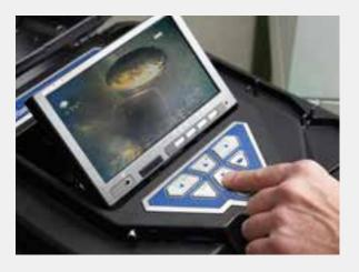
The Home button realigns the camera head to its initial position. The position and angle display indicate top and bottom of the pipe on the monitor at all times and at how many degrees the camera is being guided up or down.
